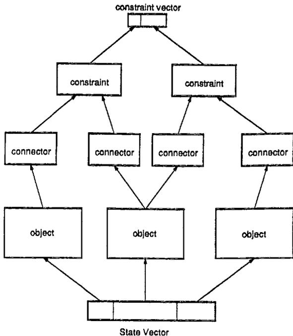
Figure 1: A schematized model. The three objects' state vectors are concatenated to form the global state vector, and the two constraints' outputs form the global constraint vector. The constraints depend on state through connectors, which represent outputs of the objects. The whole structure defines the global constraint function  $c_i(q_j)$ . Each constraint-object pair defines a block in the constraint Jacobian matrix. The block may be non-zero only when the constraint depends on the object.
