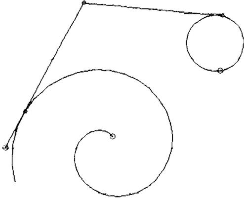
Figure 3: A model consisting of parametric curves attached by constraints. By grabbing and pulling arbitrary points on the curve, the user may move and reshape the model subject to the constraints.
